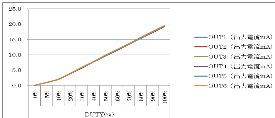
LEDVCC:5V PWM:1KHz 設定電流:19.3mA
